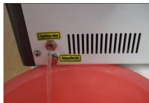
Fig 2 – water out from Overflow Hole, so tank is full
